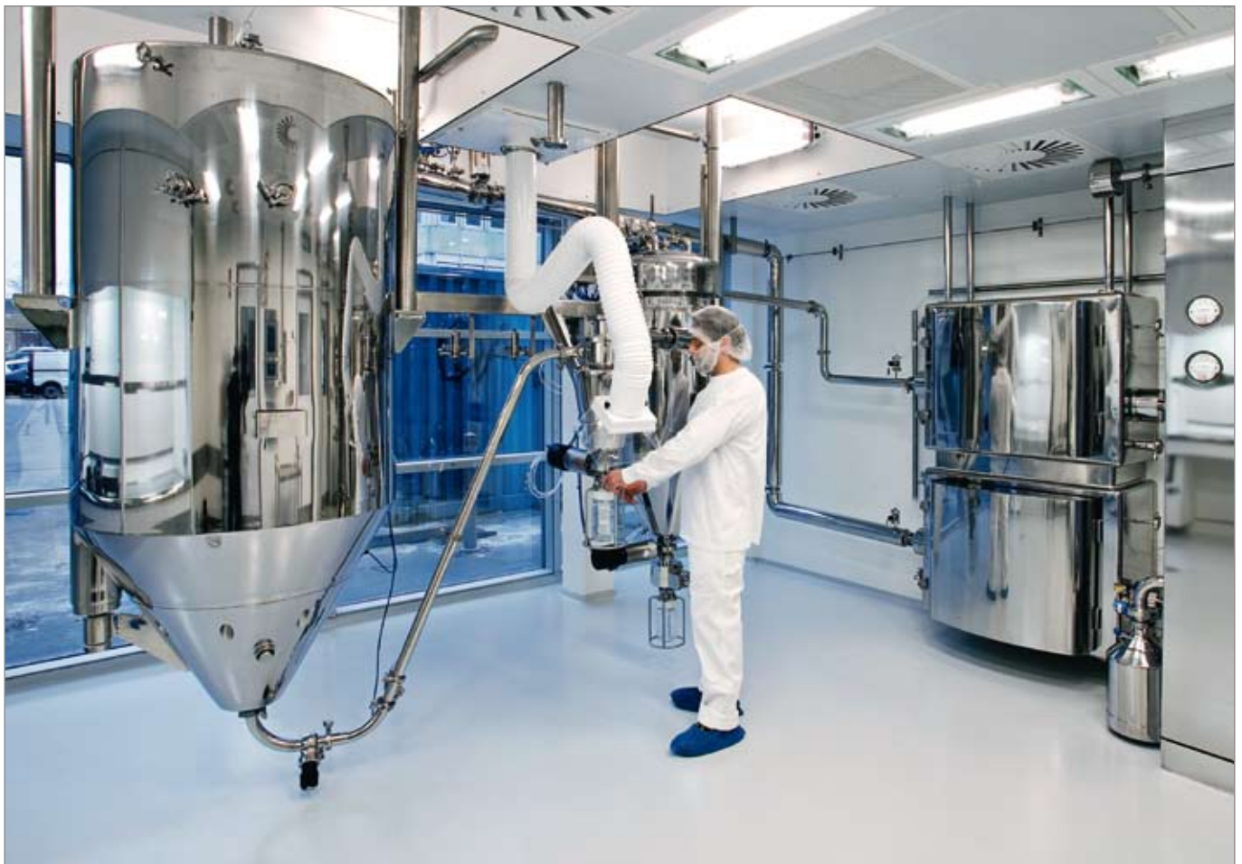
From Niro Pharma Test Station in Copenhagen: GMP suite with a PSD-1 spray dryer in closed cycle mode
