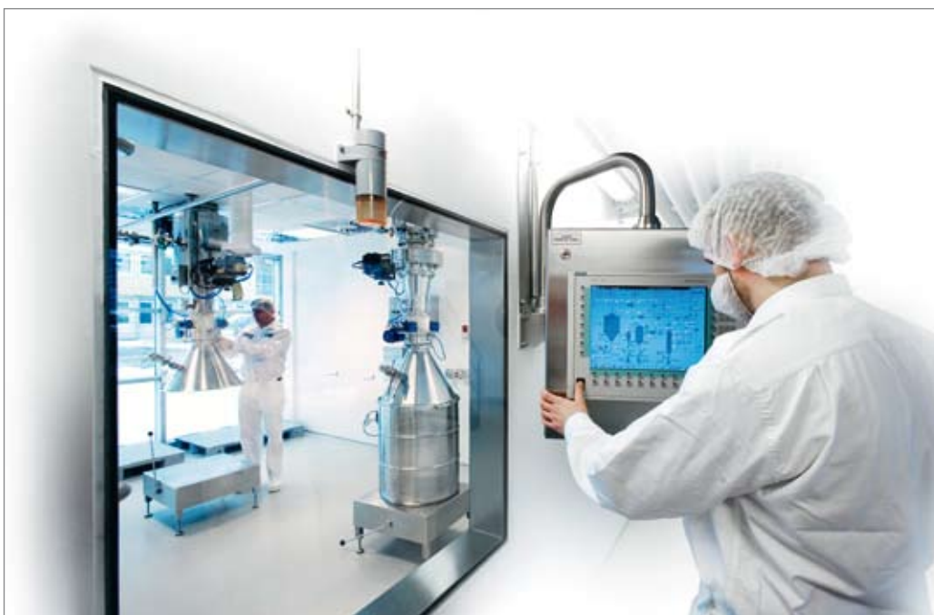
From Niro Pharma Test Station in Copenhagen: GMP facility including a PSD-4 spray dryer operating in closed cycle mode
