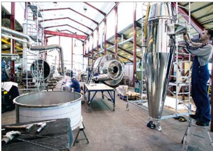
Manufacturing of drying chamber and cyclone under strict quality control
